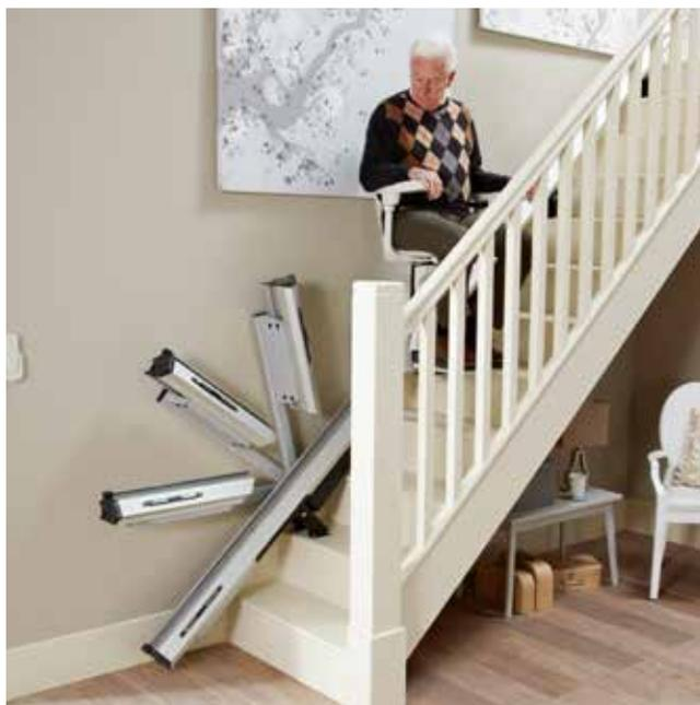
If you have an obstruction at the foot of the staircase you can choose to have an automatic powered hinge installed. Once you have used the stairlift it will return to the top of the stairs and the lower section of the rail will fold away, leaving the bottom of your staircase clear.
